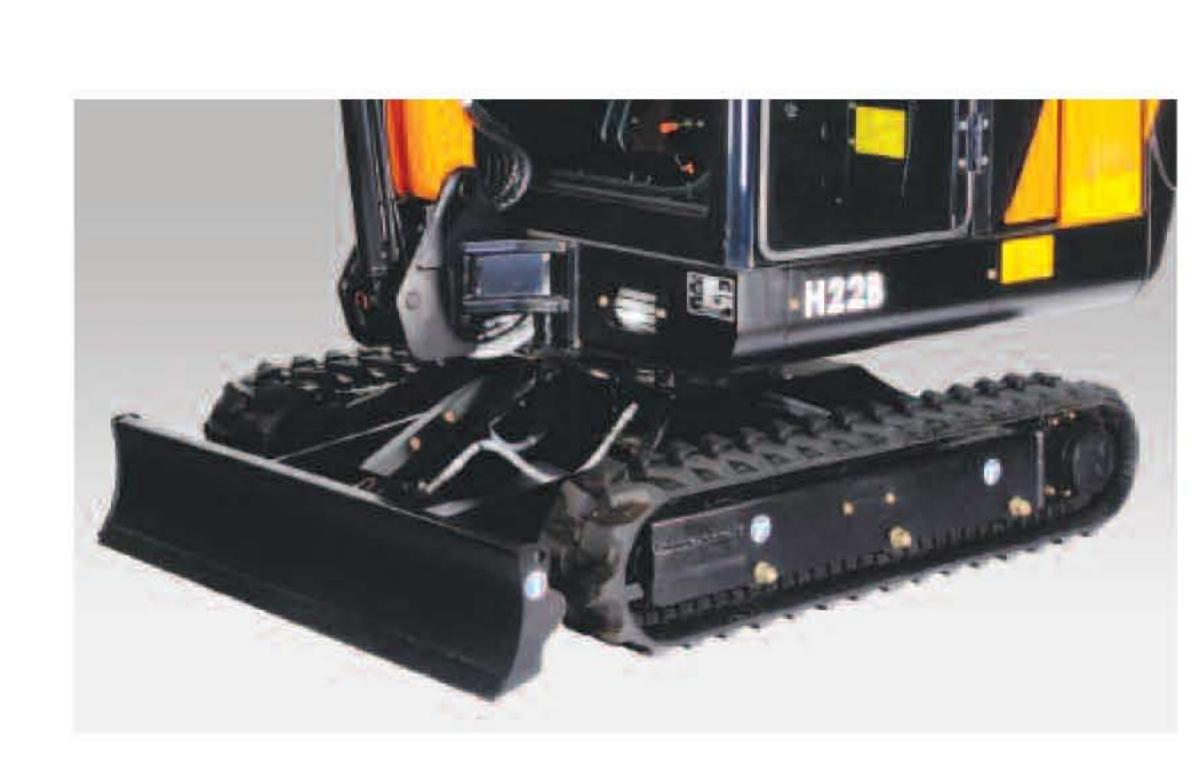
Long 'X' track frame with generous ground clearance provides strength and versatility in all conditions.
