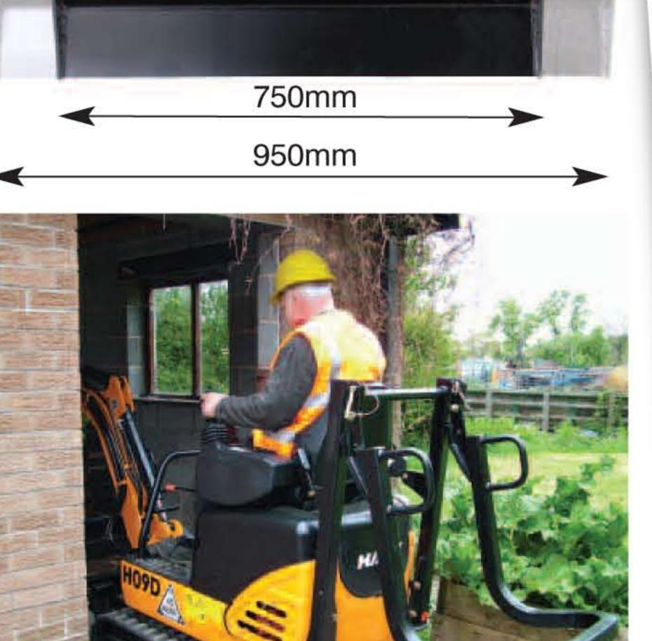
Combination of hydraulically retractable tracks and folding ROPS enables the HO9D to pass through narrow openings with low headroom clearance.
